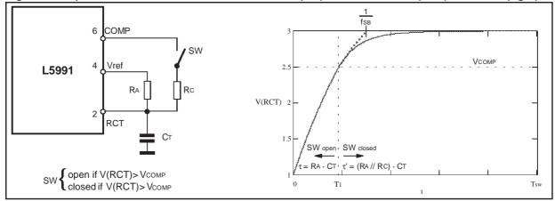
As long as the oscillator voltage V(RCT) is less then V<sub>COMP</sub>, D1 is reverse-biased (SW is open) and only R<sub>A</sub> contributes to the time constant  $\tau$ ; moreover, the asymptote of the exponential curve is the reference voltage V<sub>REF</sub> (5V). When V(RCT) equals and exceeds V<sub>COMP</sub>, D1 is forward-biased (SW is closed), then R<sub>C</sub> goes in parallel to R<sub>A</sub> to determine the time constant  $\tau$ ' and the asymptote will be changed to:
