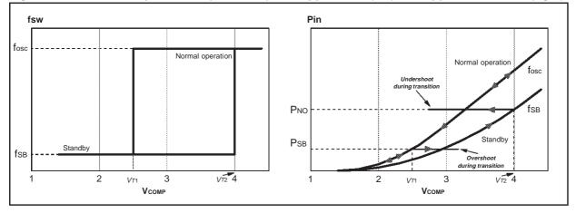
Figure 1. L5991's Standby function operation: f<sub>sw</sub> vs. V<sub>COMP</sub> locus (left) and V<sub>COMP</sub> vs. P<sub>in</sub> locus (right).
